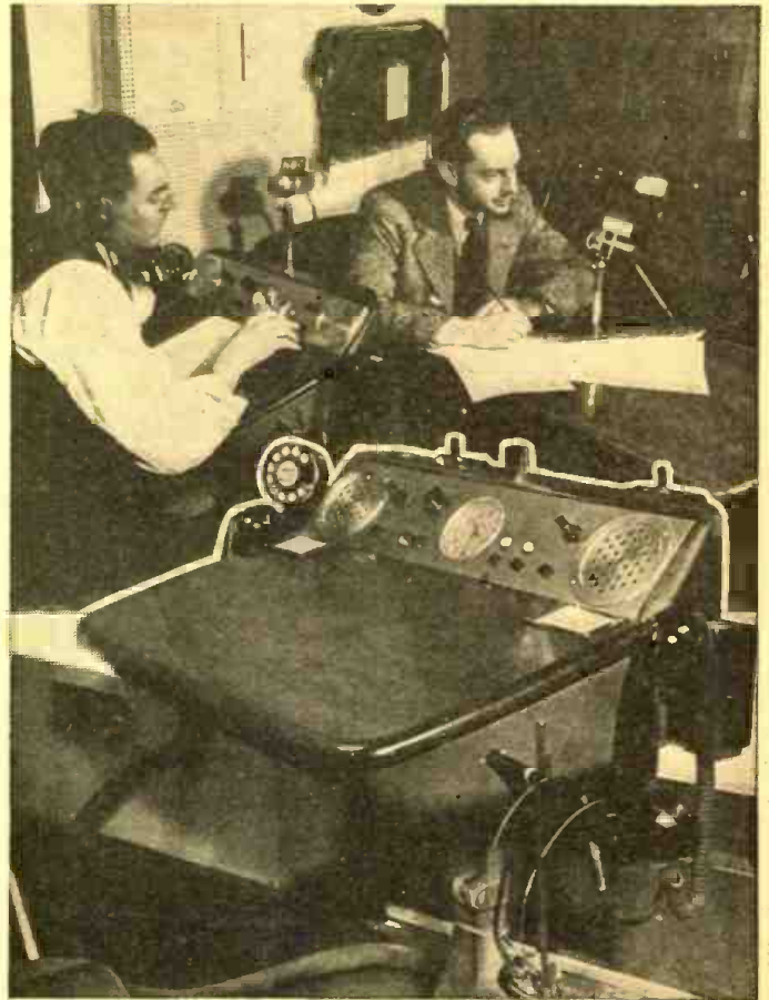
Picture at right shows an engineer at the new "school room" control desk, monitoring a broadcast by John W. Vandercook. Inset at the bottom is a closeup of the desk. Notice dial phones at both ends of desk with a loudspeaker next to each. Clock at center aids in timing programs.
